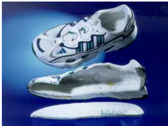
Fig. 23: Adhesive bonding technology in shoe manufacture - adhesively bonded laminate construction of a sports shoe
