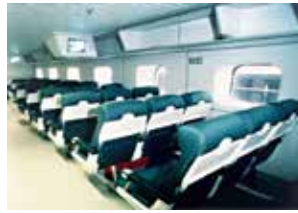
Fig. 14: Shipbuilding - The polycarbonate passenger window panes and the rows of seats (picture in the middle and one on the right) are adhesively bonded in place. 24
