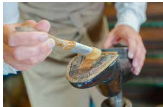
Fig. 24: Adhesive bonding technology in shoe repair 37
